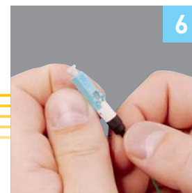
Slide the boot onto the connector
