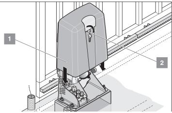
Mount the cover (2) and push it down. Turn key (1) 90° in anticlockwise direction and remove it.
