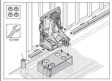
• Mount the operator on the console and connect the cables.
