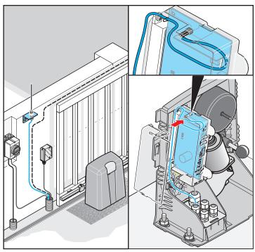
· Connect external antenna to the respective adapter.
