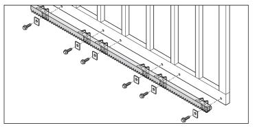
Secure rack to the gate, using appropriate fixtures (e.g. supplied screws). Secure rack at all six fixing points to the gate.
