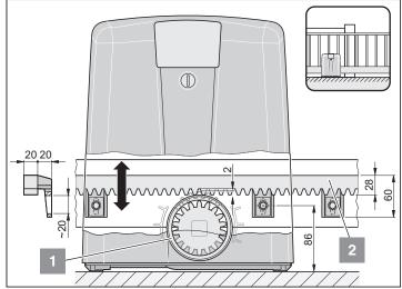
Push the gate several times back and forth. Ensure that the gear rod (2) touches the mounting ring (1) along its entire length.
