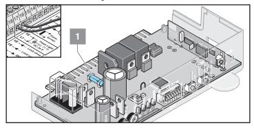
1. Fuse for connection of warning lamp 1, terminal 16 + 17
