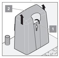
• Turn the key (1) 90° in clockwise direction and lift off the cover (2).
