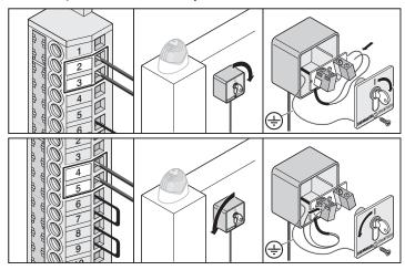
Install key switch box at a suitable location that can be easily accessed.
