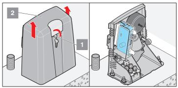
• Turn the key (1) 90° in clockwise direction and lift off the cover (2).
