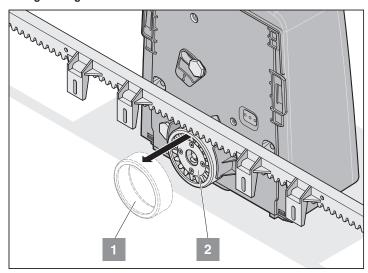
• Pull the mounting ring (1) from the gear (2).
