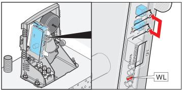
• Press and hold buttons (1 + 2) until the LED (warning lamp) is off † "WL" LED off - force values deleted. Release the buttons (1 + 2).
