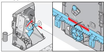
Pull lever (1) and swivel the motor (2) to the right, until it engages with a loud clicking sound. Release the lever (1) while the motor is engaging.
