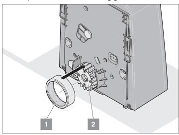
• Push the mounting ring (1) on to the gear (2).
