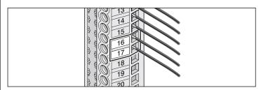
Terminal 16 + 17 unregulated DC 24 V (max. 34 V) 25 Watt, max. 1 A Protected with 1 A fuse, fast-acting.
