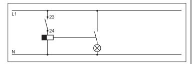
Example: Staircase lighting with automatic switching system
