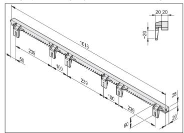
Mount the first rack at the opening edge of the gate. To mark the holes for the securing bolts, position the respective rack over the toothed wheel.
