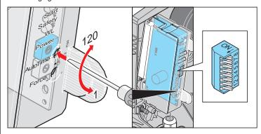
The GATE OPEN time can be adjusted at the potentiometer:
