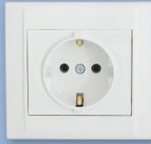
42001028 TOPRAKLI PRİZ SCHUKO SOCKET OUTLET Gerilim / Rated Voltage 250V Akım / Rated Current 16A Koruma Derecesi / Protection IP20
