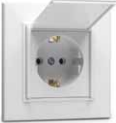
Kapaklı Topraklı Priz Earthed Socket-Outlet With Lid 56001029 16 A, 250 V~ IEC 60884-1
